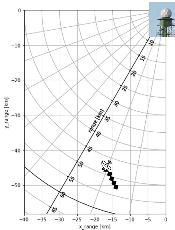
Figure 2: Approximate projection of the satellite slant path on four radar bins shown by dark color. The first top left of these four black bins shows the location of the UT as well as the collocated rain gauge. The Southwest Germany DWD radar is about 50 km away from the UT.
