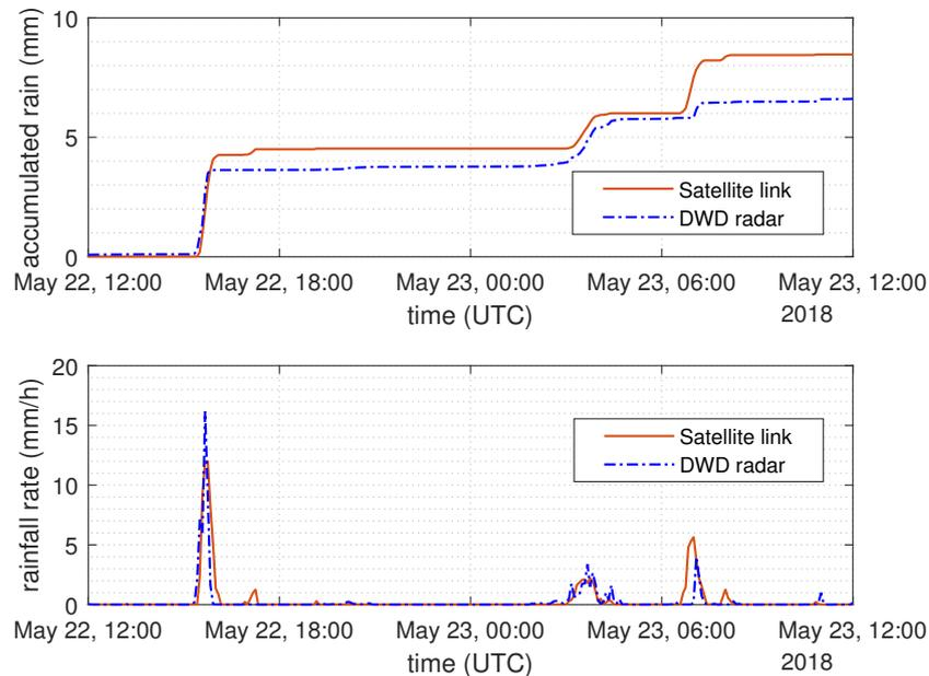
Figure 5: Rain accumulations during 24 hours from 1200 UTC on 22 May 2018 till 1200 UTC on 23 May 2018 as observed by the Southwest Germany DWD radar (dashed blue line) and satellite link (encircled UT in Fig. 3) using our proposed algorithm (solid red line).
