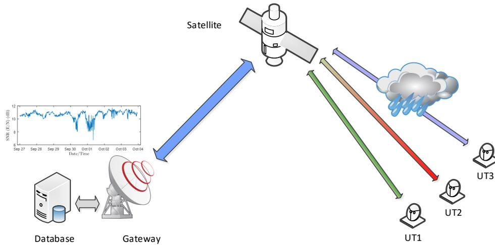
Figure 1: Architecture of a Broadband Satellite Communication Systems. The C/N data of the FWD and RTN links are collected by the gateway and stored at a database. We use these data for rainfall estimation.
