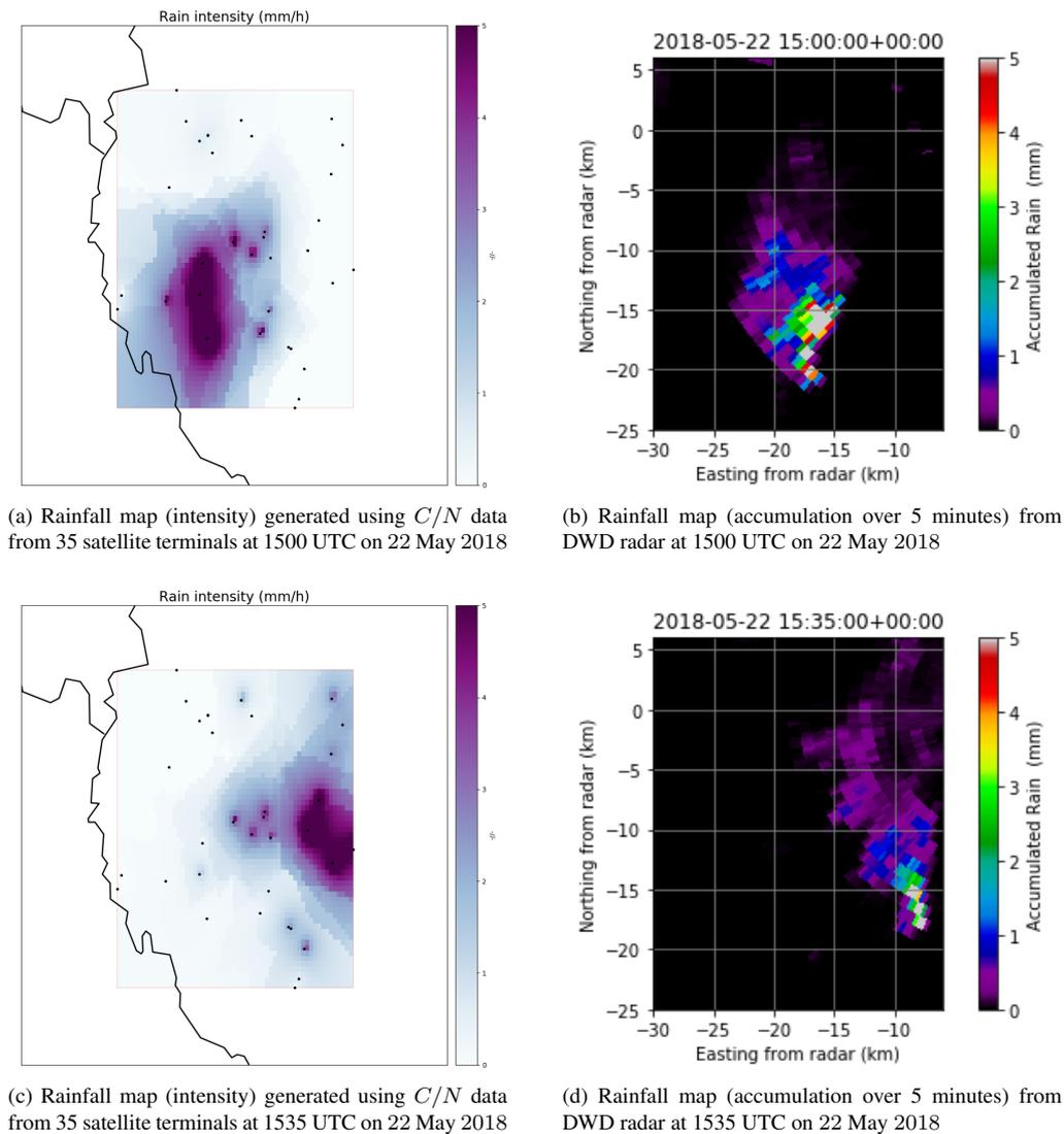
Figure 6: Comparison of the rainfall maps produced by our LSTM-based algorithm and the nearest DWD radar at two different intervals for a storm passing over Southwest Germany on 22 May 2018 UTC.
