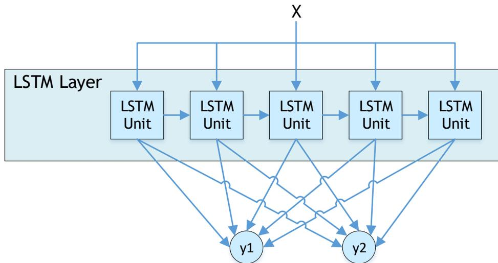
Figure 4: Structure of LSTM network for rain/dry classification.
